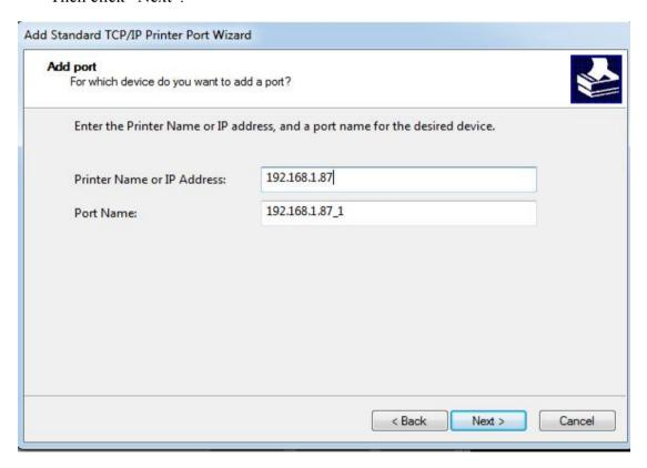
Enter the IP address of the printer Ethernet port, Factory default IP is "192.168.1.87".
