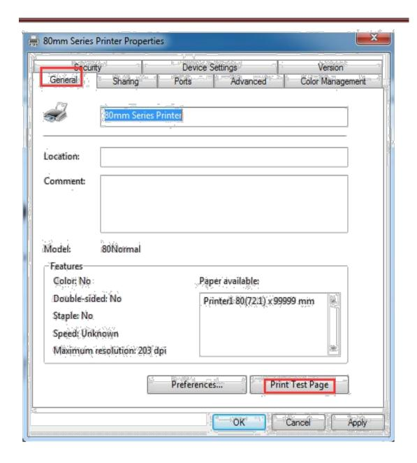
Click "Print Test Page", the printer will print test page, which means the printer has been connected with computer successfully and the port configuration is correct.
