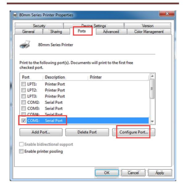
Select available computer COM port, such as "COM1" as the above picture, and then click "Configure Port" to set the detailed parameter.
