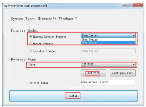
Select the Printer Model and available computer port, such as "USB PORT the picture, then, click "Install".
