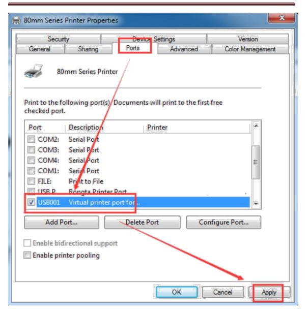
Select available computer USB communication port, such as the above picture shows "USB001", and then click "Apply" to finish the configuration.
