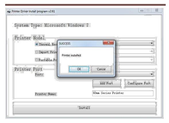
Select "OK", and then click "Exit". Wait until it shows the below picture, it means, the printer driver has been installed successfully.
